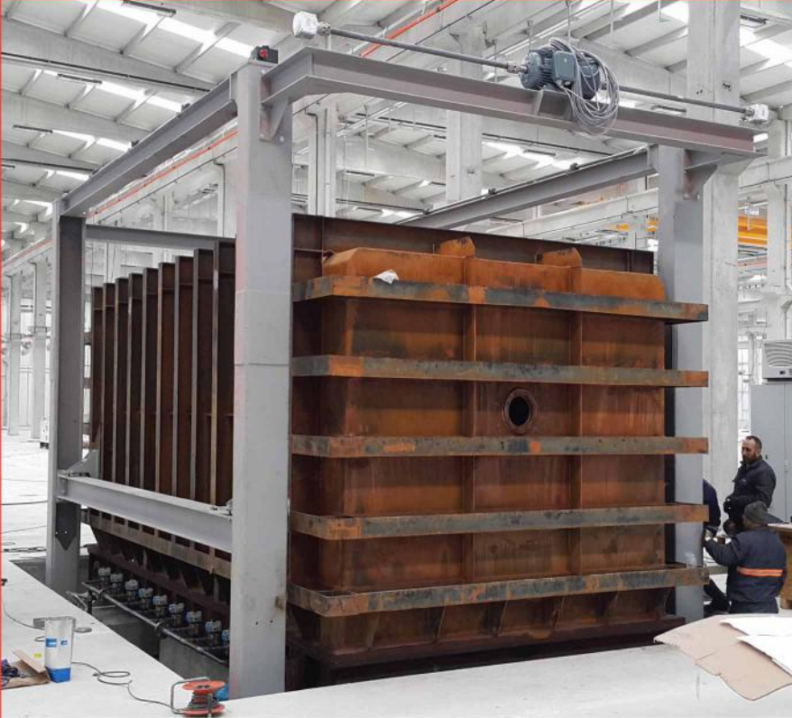
Vacuum Chamber, Germany
