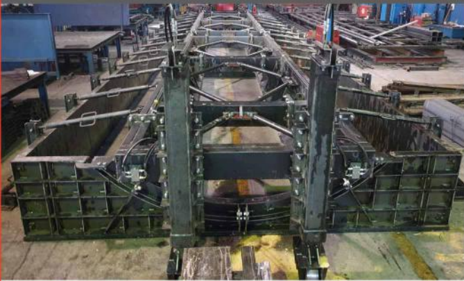
Invert Formwork, Iraq
