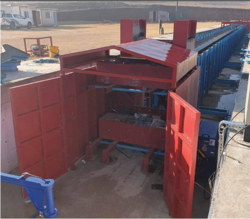
Baban Autobahn Bridges, Sulaymaniah, Iraq Turnkey solution from formwork to all accessories like vibrators, steam chamber, pre-stressing eqips etc.
